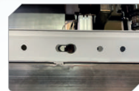
MILLING RESULTS TO FIT THE HANDLE
