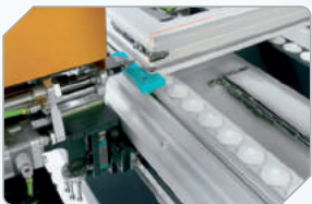
SENSORS TO PREVENT THREAD STRIPPING
